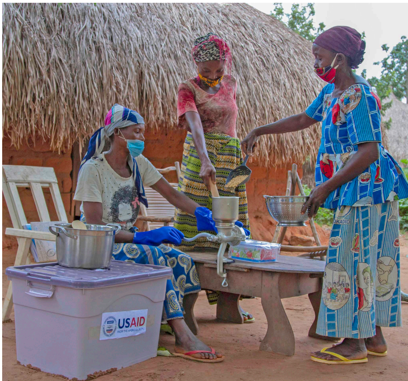
Members of a producer organization use a SoyaKit to process soybeans into soy beverage. [Photo CRS]
