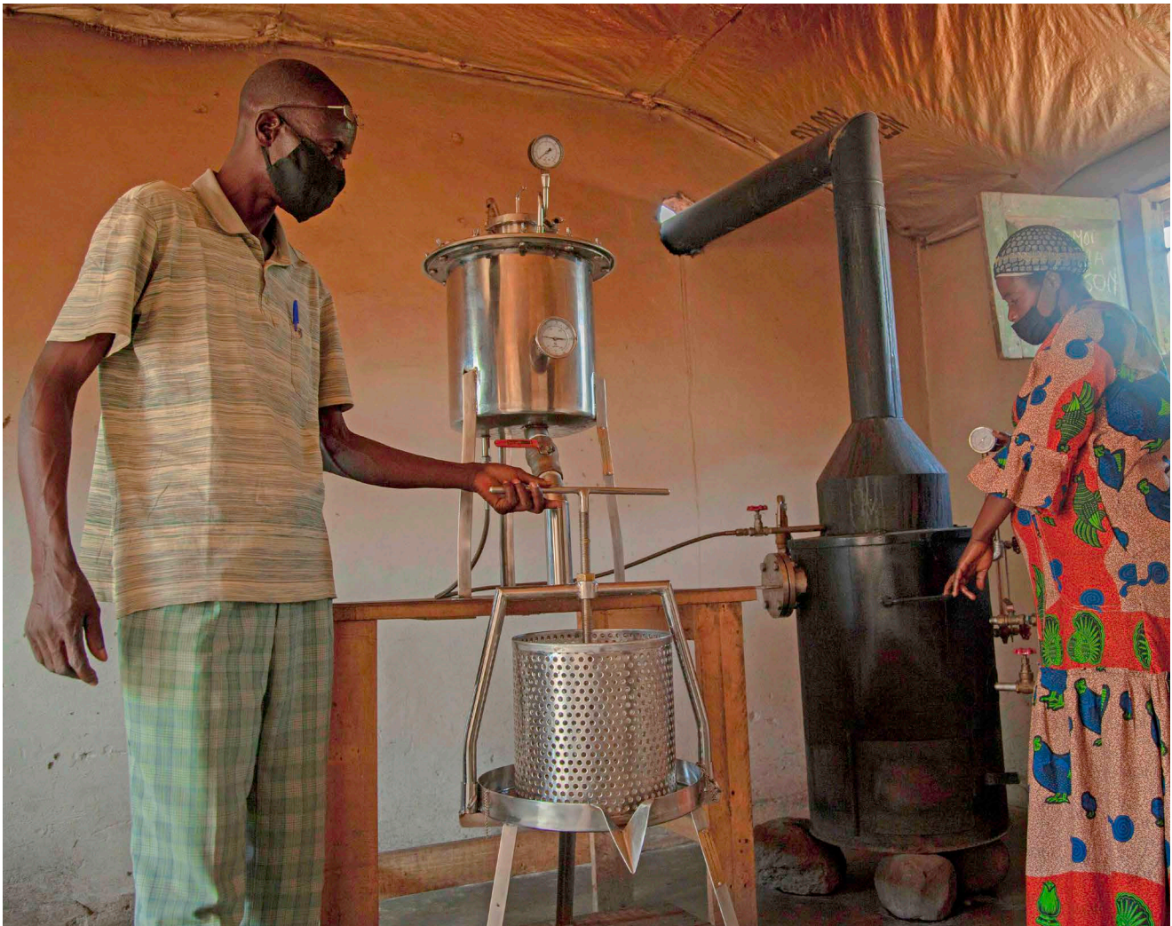
Members of a producer organization employ a VitaGoat to process soybeans. [Photo CRS]
