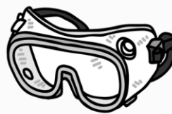
Goggles and anti-dust or respirator masks for handling items that can affect sight or respiration (e.g., flours, timber, cement, sand, packets of insecticide or chlorine)
