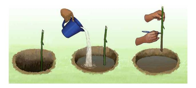
We will now start the soil drainage test. We will use one of the holes to test water drainage. Place a marking stake or straight tree branch into the hole. Fill the hole with water, mark on the stick the top of the water line. Use a watch or a timer on your phone to track time.
