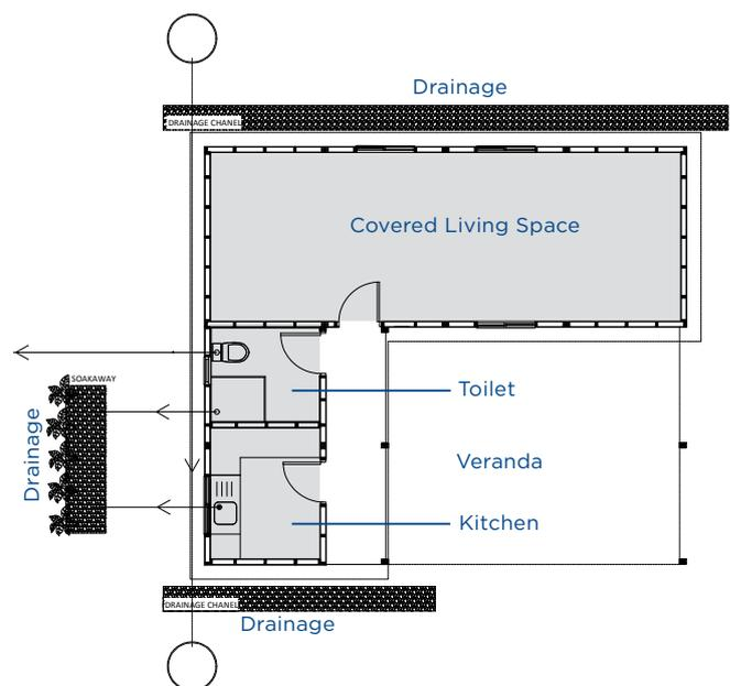
The project built shelters of different sizes, to adapt to the different family sizes. Shelters included a bedroom/living area, a toilet, a kitchen and an open veranda, that could be used to expand the covered space, by adding walls. People had to take care of the external sanitation system, e.g. septic tank.
