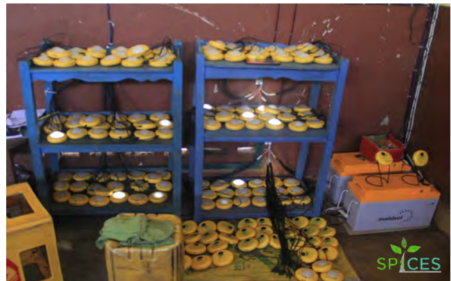
Arthur's Jiro Ve solar lights. Each morning he collects and charges the lights and then redistributes them to his customers before sunset.
