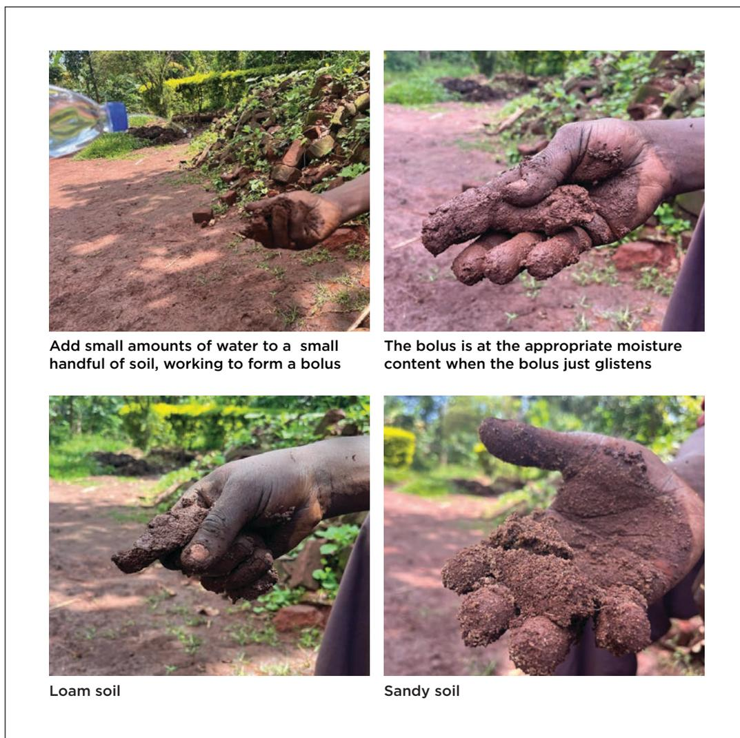
**Figure L4.2.** Simple methods for testing soil texture
