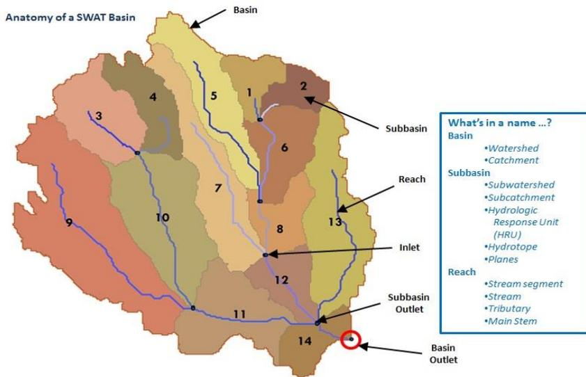
Figure 2. Common terminology used in describing parts of a basin. SWAT divides a basin into subbasins, which can be further divided into individual hydrologic response units (a unique combination of land cover, soils, and topography). Sometimes you may hear alternative names (bullet points) used.
