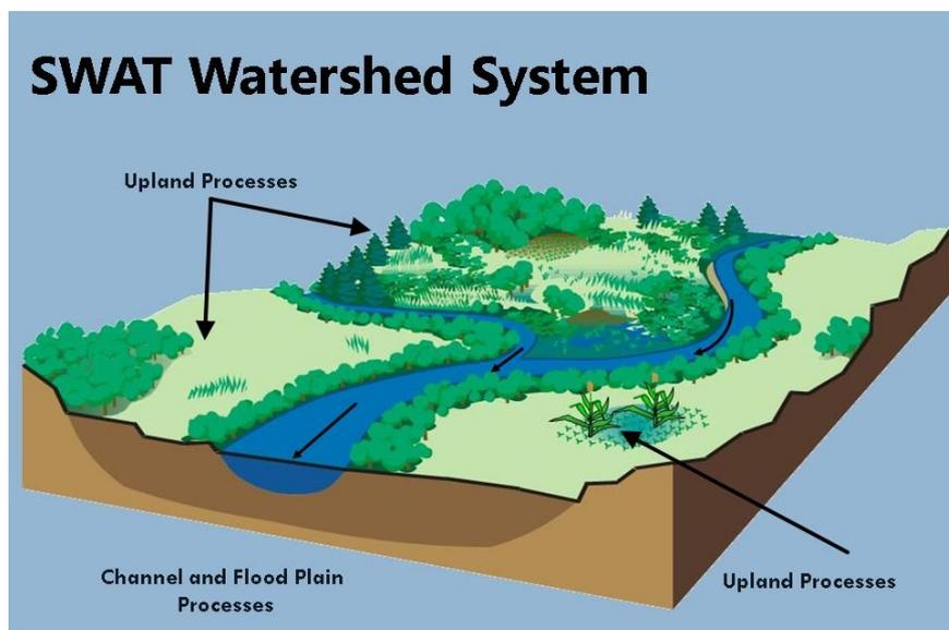
Figure 1. SWAT can model upland and channel processes, allowing users to also assess processes such as erosion (using the Modified Soil Loss Equation), flood routing, sediment routing, evapotranspiration, crop growth, and others.
