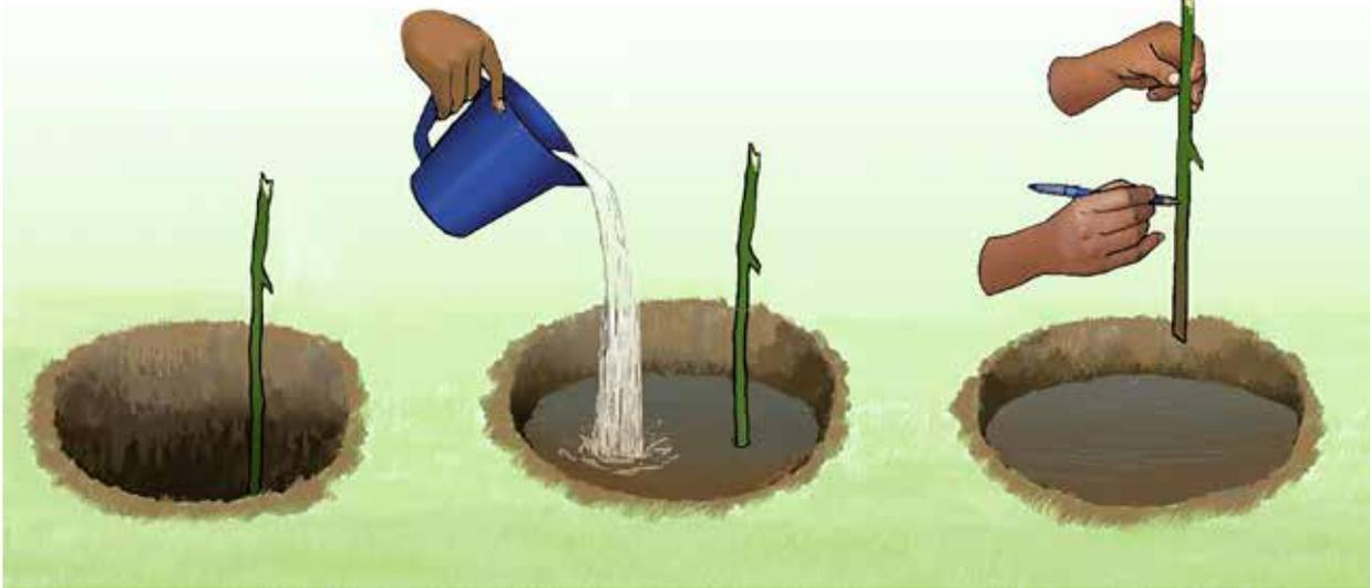
We will now start the soil drainage test. We will use one of the holes to test water drainage. Place a marking stake or straight tree branch into the hole. Fill the hole with water, mark on the stick the top of the water line. Use a watch or a timer on your phone to track time.
