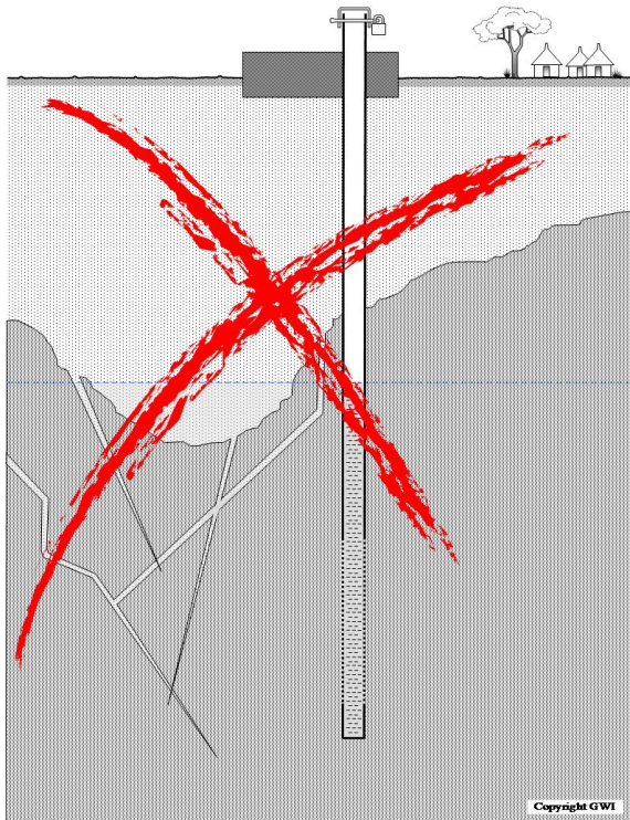
Figure 15: wrong siting in fractured rock
