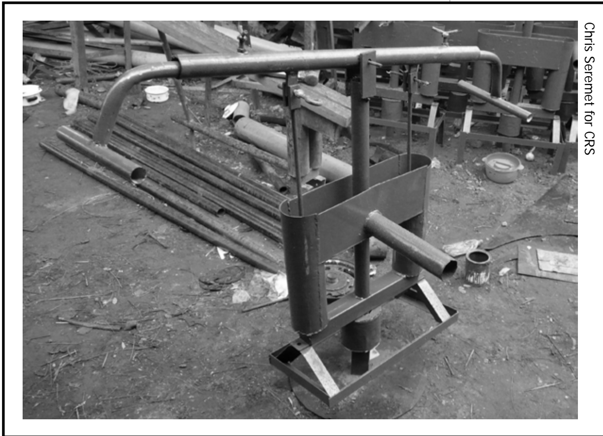
A locally-manufactured suction pump in Niger.
